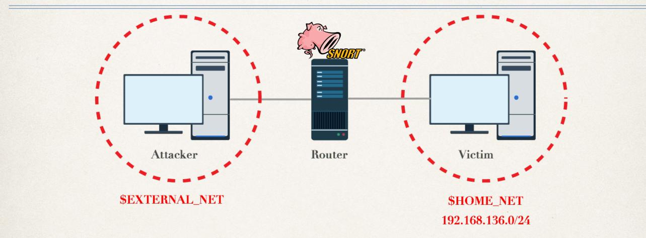
Snort is installed on the router on the border of our HOME\_NET
