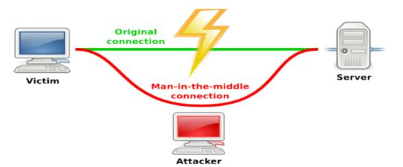
In this technique an attacker is in the middle of a connection between two devices and sniffs the packets that are exchanged. Then it can partially or totally modify those packets to its will.
