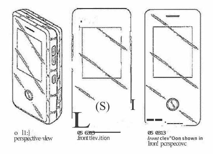
The planar front surface of **0546,313** shares the same basic design characteristics with the claim in that the front perspective view shows 1- A flat panel with an outer rectangular shape having substantially the same aspect ratio. 2- Four evenly
