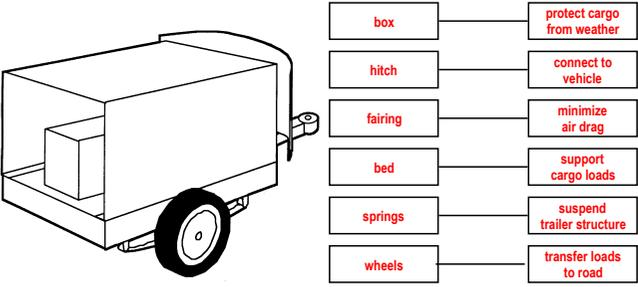
The diagram shows a trailer with a box, hitch, fairing, bed, springs, and wheels. Lines connect these components to their functions:
