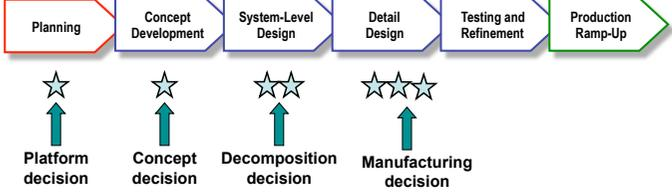
The flowchart shows a sequence of six stages: Planning, Concept Development, System-Level Design, Detail Design, Testing and Refinement, and Production Ramp-Up. Below the first four stages are decision points: Platform decision (1 star), Concept decision (1 star), Decomposition decision (2 stars), and Manufacturing decision (4 stars). Arrows point from each decision point to its corresponding stage.
