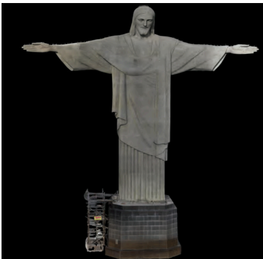
FIGURE 34: PIX4D POINT CLOUDS OF CRISTO REDENTOR FROM SENSOR DATA
