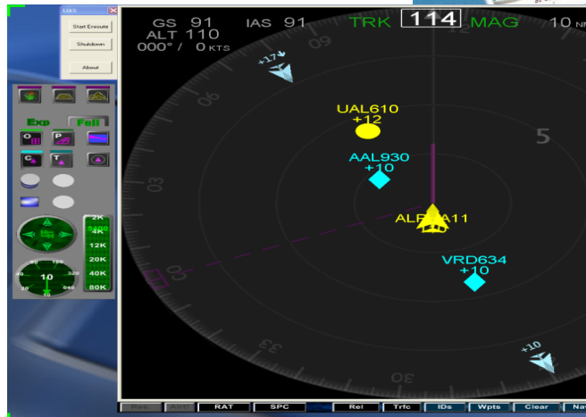
NASA's UAS cockpit situation display with TCAS advisories
