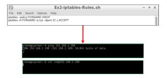
• Test on the VM Green if you can still ping or connect with ssh on MV Red. Now it is impossible to ping the VM Red, but also to connect with ssh. This
