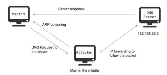
In order to make this attack work on a single physical machine, a little tweaking was necessary and a 1 second network delay has been added to the packet output by the server VM, to prevent it from answering before the attacker could.
