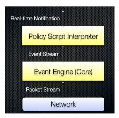
A simple schematic representation of the software structure and behaviour (on the left).
