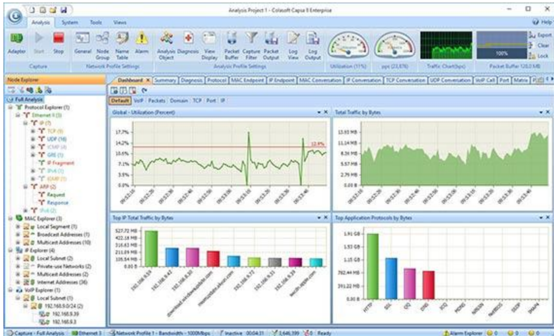
Fig 16: Show different types of traffic measure in Bar chart using Capsa Network Analyzer
