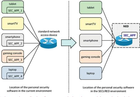
Moving security applications from user terminals to the network (network edge device (NED)) - HINT
