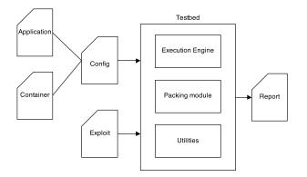
Figure 1: Overview of the testbed architecture
