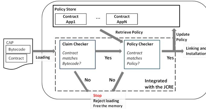
**Fig. 2.** *The Security-by-Contract workflow for loading.*
