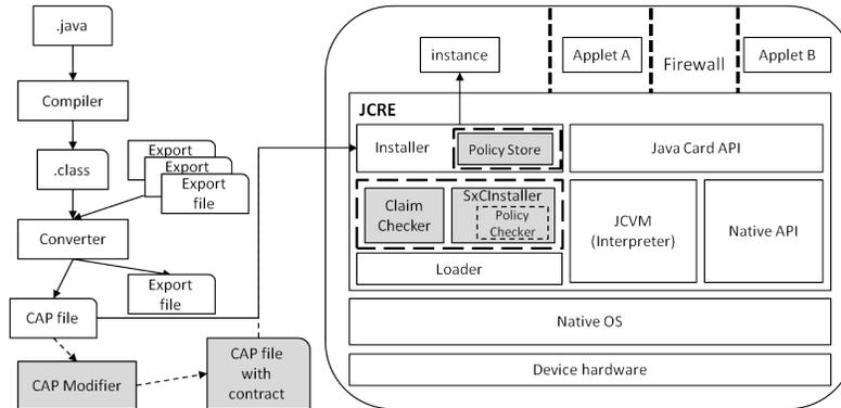
**Fig. 1.** The Java Card architecture and the loading process. The white components and data structures belong to the standard Java Card platform. The grey components and data structures are additions introduced by the SxC scheme. The dashed lines denote the changes to the loading process.
