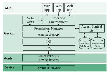
Fig. 1: The Firefox OS architecture [2]
