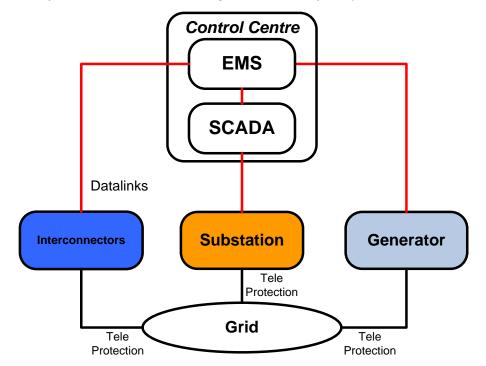
Figure 2 - Data links between the Control Centres, Interconnectors, Generators and Substations
